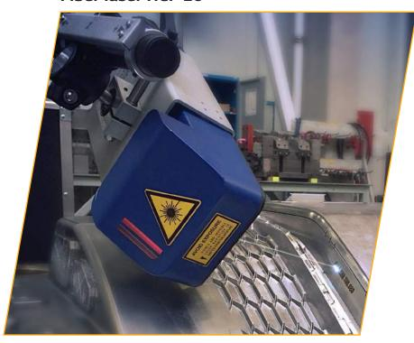
New way of laser head clamping to optimise its rotating to work position. Improved focusing of laser head on the working area by using two red points.
